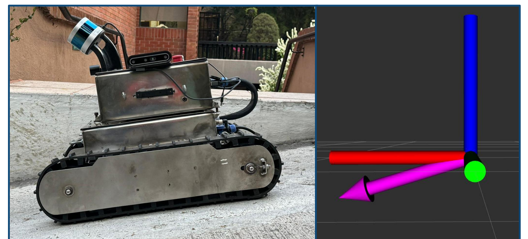
Fig 5. Inclination measurements performed using IMU data.
