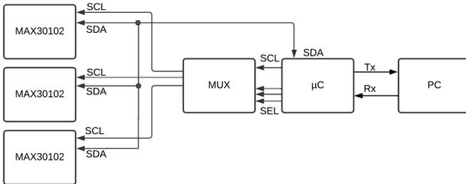
Fig. 2. NIRS system acquisition diagram block for the three optodes used to prepare the dataset.
