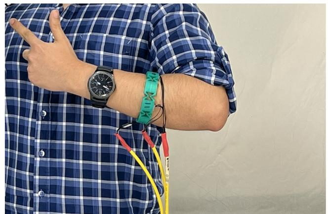
Fig. 1. The NIRS acquisition system placed on the forearm of one of the volunteers. The bracelet facilitates the location of the three optodes in three specific groups of muscles.
