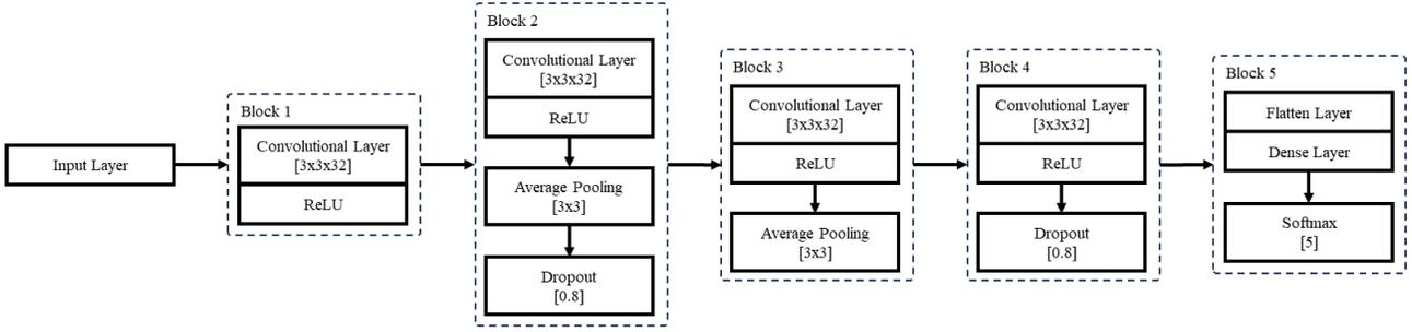
Fig. 4. CNN model architecture used for hand gesture classification for both EMG and NIRS-based methods.
