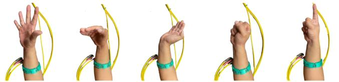
Fig. 3. Gestures performed by the subjects. From left to right: Hand Open (HO), Wrist Flexion (WF), Wrist Extension (WE), Hand Close (HC), and Index Finger Extension (IFE), respectively.
