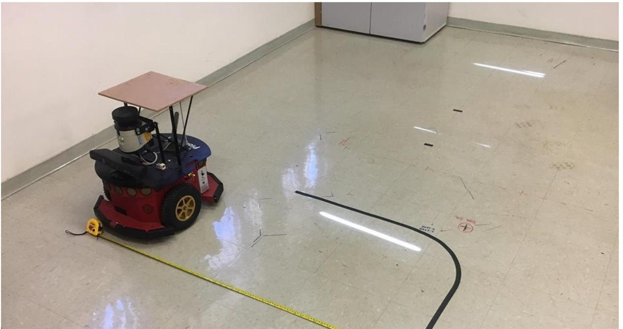
Figure 2.1 – Pioneer P3DX differential wheeled robot from Adept Robots into an indoor environment.
