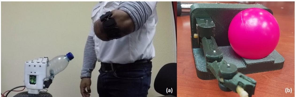
Figure 6.1 – (a) A limb-impaired volunteer tests the Galileo Hand holding a water bottle. (b) The test bed used to standardize the experiment iterations of each finger interacting with a small plastic ball.
