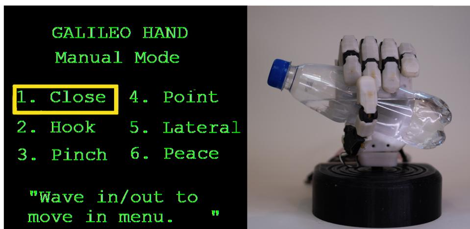
Figure 2.9 – Galileo Hand’s graphical menu (left) and the prosthesis performing the action “Close” (right).
