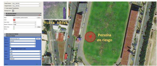
Fig. 4. Dashboard based on MapViz to see the markers and the drone position
