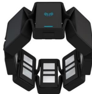
The Myo armband promptly recognizes 6 different hand gestures, wave in, wave out, double tap, fist, spread fingers and rest gestures. In this work, it was used only three of the six gestures, wave in, wave out and spread fingers, as shown in Figure 6. The use of this gestures is associated with the control strategy and are described in details in the next section.
