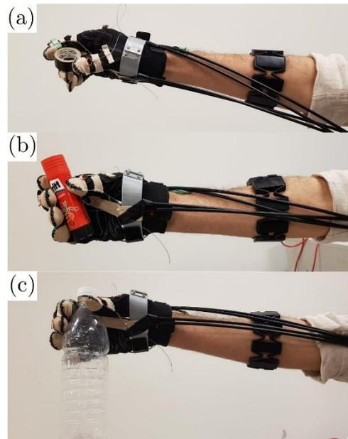
As can be seen, the implemented differential mechanism allows the actuated fingers to easily adapt to the objects surface, as was expected. Moreover, it is worth to mention that as a result of using the differential mechanism, it is possible to execute the pinch grasp motion.
