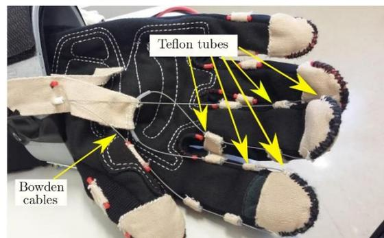
As the glove's fabric is flexible, thimble-like caps made from inextensible fabric were stitched at the fingertips. These act as anchor points for the tendons, providing a firm support for the U-shaped Teflon tubes rounding the fingertips. Moreover, they allow the fingers to move in the intended direction (finger extension/flexion) when tendons force the thimbles.
