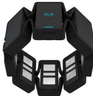
The Myo armband promptly recognizes 6 different hand gestures, wave in, wave out, double tap, fist, spread fingers and rest gestures. In this work, it was used only three of the six gestures, wave in, wave out and spread fingers, as shown in Figure 6. The use of this gestures is associated with the control strategy and are described in details in the next section.
