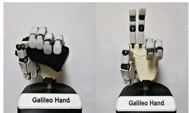
Fig. 9. Galileo Hand is performing power grasping and the peace sign.
