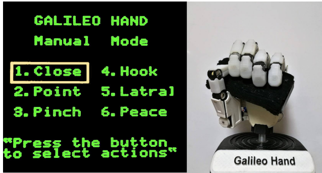
Fig. 7. Graphical UPI on Galileo Hand performing power grasping.
