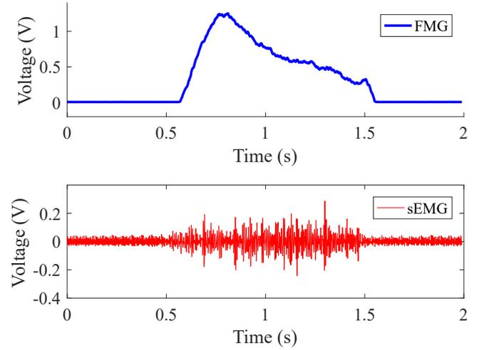
Fig. 5. Comparison between optical-fiber FMG and filtered sEMG.
