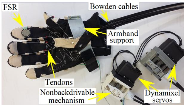
Fig. 2. Wearable robotic glove and its components.
