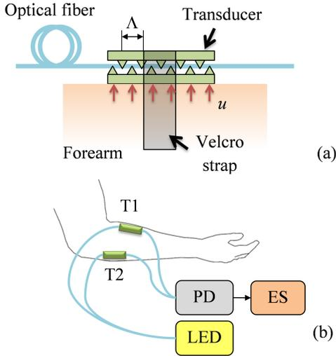
Fig. 3. FMG sensor system: (a) microbending transducer representation; (b) measurement setup. Note:  $u$ : displacement caused by muscles activity; PD: photodiode; ES: embedded systems. T1 and T2: transducers.
